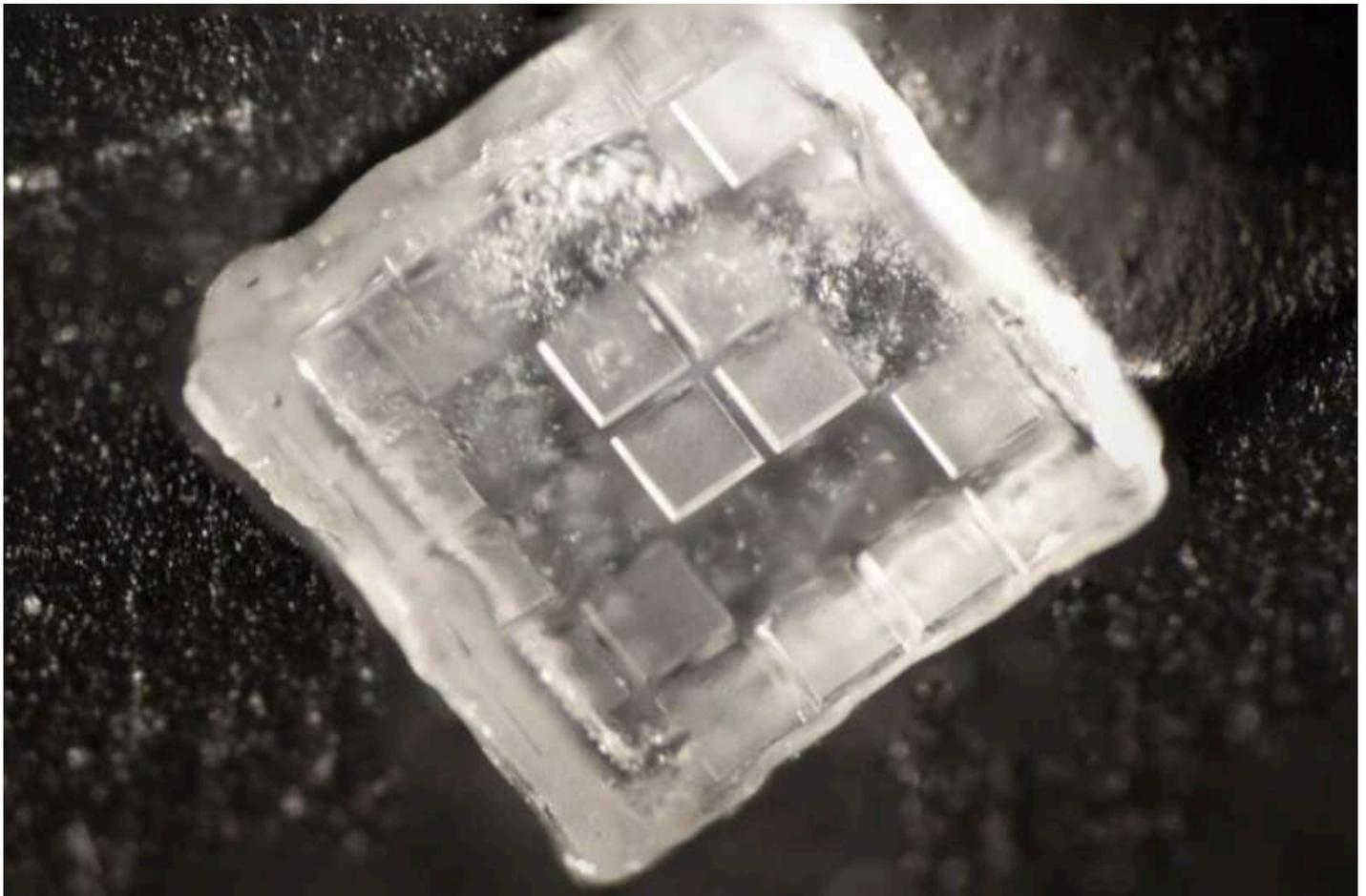
A microscale diffuser on the transducer that produces the ultrasound waves is built based on the Schroeder diffuser—the best sound diffuser mathematical models can provide. This is the same math that is used to design concert halls so that every audience member can hear music perfectly. Credit: University of California San Diego
